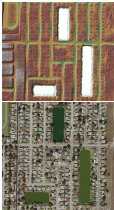
Figure E.1a. Top view: Topobathy lidar derived DEM that contains lidar voids within stormwater retention ponds in Tarpon Springs, FL. Bottom view: Orthoimage of the same area. Such retention ponds are used to manage stormwater runoff to prevent flooding and downstream erosion, and to filter pollutants to improve water quality in adjacent rivers, streams, lakes, or bays. Image courtesy of NOAA.
