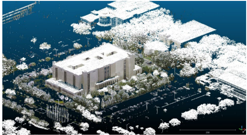
Figure E.23a. Hillsborough County Florida aerial lidar fused with terrestrial scanned data of the library and other buildings at the University of South Florida. Image courtesy of USF. Many planners develop 3D virtual models of the built environment for urban and regional planning and visualization of proposed construction projects
