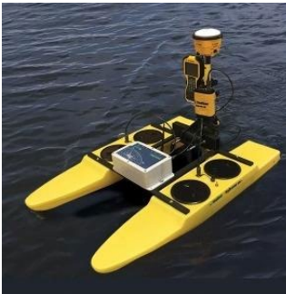
Figure L.47. The HydRone is ideal for hydrographic surveys of lakes and ponds. Image source: Seafloor Systems
