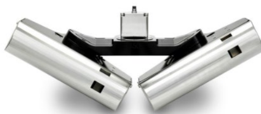
Figure L.37. The RESON SeaBat Integrated Dual Head T20/50-R is a sonar system that produces 1,024 beams per ping, frequency from 200 to 400 kHz, allowing for swaths on both sides of small boats in shallow water. Image source: RESON
