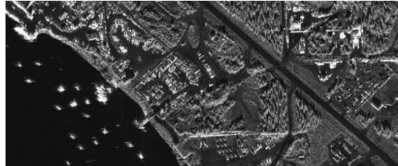
Figure L.17. Type-I 25-cm ORI flown from 18,000 feet
