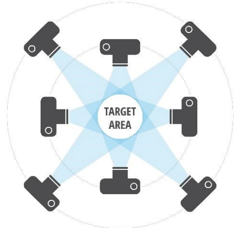
Figure L.10. With SfM, highly redundant image overlap allows for self-calibration of non-metric cameras and mapping in a local coordinate system. Surveyed GCPs are normally added to improve map accuracy. Image source: Dewberry
