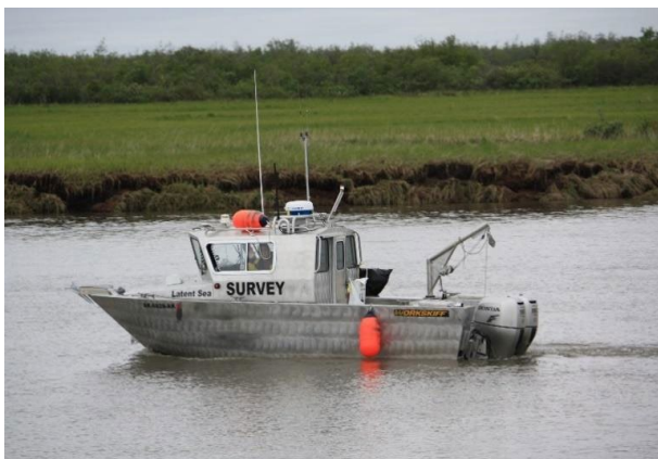
Figure L.43. Typical crewed hydrographic survey vessel used for mapping of inland bathymetry. Image source: TerraSond
