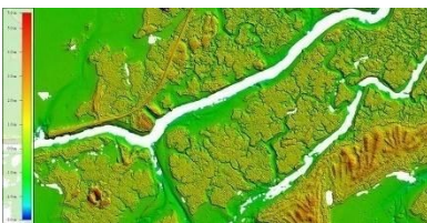
Figure L.31. Topobathy lidar mapped portions of the river, but not the deeper tannic waters with mucky bottom. Image source: Dewberry
