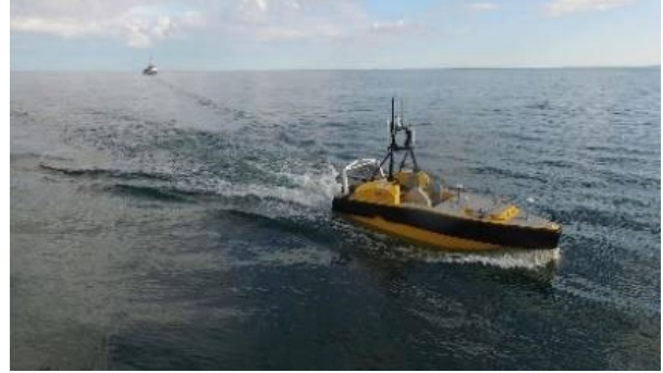
Figure L.45. With the mothership in the background, the CW5 is a proven USV platform for nearshore bathymetric surveys with a variety of sonar sensors. Image source: L3-Harris
