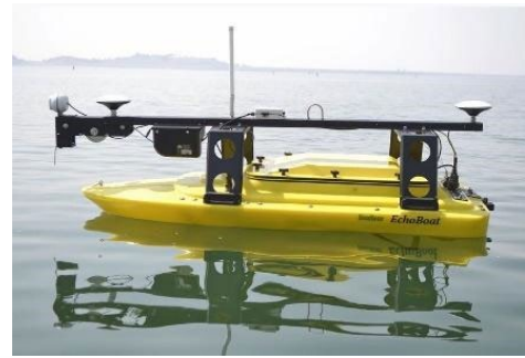
Figure L.49. The EchoBoat-160 is advertised for MBES surveys in “choppy inland waters” but not for ocean waves. Image source: Kuker-Ranken
