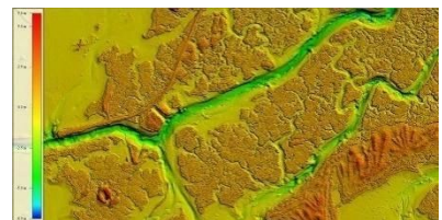
Figure L.33. By merging the two datasets the entire topographic and bathymetric surface was mapped seamlessly. Image source: Dewberry
