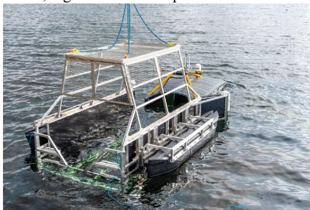
Figure L.53. XO-LARS (Launch and Recovery System) and XO-450 ASV during recovery. Image source: XOCEAN
