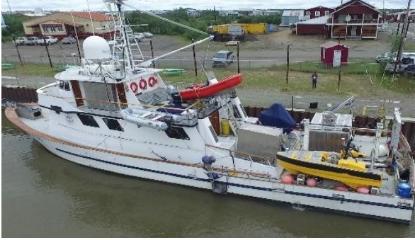
Figure L.44. Larger vessel (mothership) used for traditional MBES surveys in deeper water and CW5 USV (yellow) used for shallow-water surveys. Image source: TerraSond
