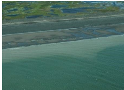
Figure L.24. Water turbidity can severely limit the depth to which topobathy lidar can map nearshore bathymetry. Image source: Alaska ShoreZone imagery
