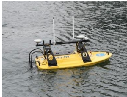
Figure L.48. Similarly, the Z-Boat is not powered to operate in waters with waves and strong currents. Image source: Teledyne Marine
