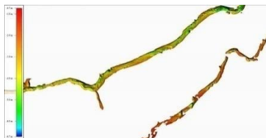
Figure L.32. Multi-beam sonar mapped the deeper parts of the river not mapped with topobathy lidar. Image source: Dewberry
